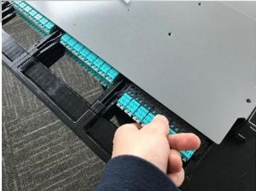
Module Box Insert/Remove from Front
